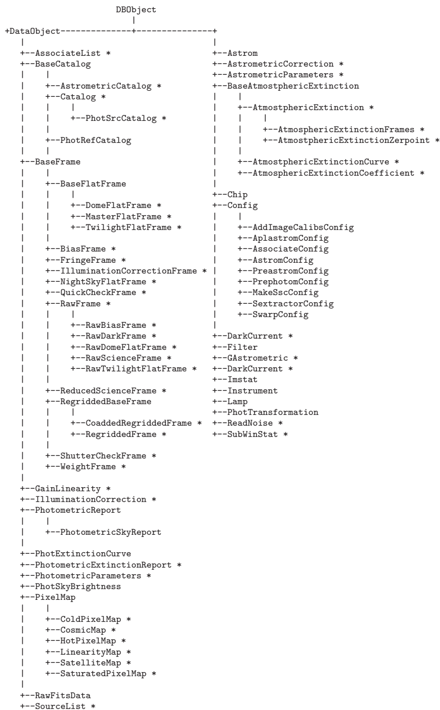
Figure 4.1: The class hierarchy of Astro-WISE. Asterisks (*) mark object that have a make() method
