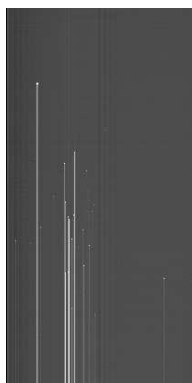
Figure 13.1: BiasFrame containing several bad columns of hot pixels.
